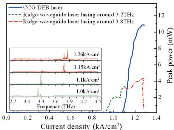
FIG. 3. Comparison of the LI characteristics of a CCG DFB QCL and a ridge-waveguide laser at 78 K. The CCG DFB laser operates only at 3.77 THz, whilst the ridge laser operates at  $\sim 3.2$  THz (green portion of the LI curve) and  $\sim 3.8$  THz (red portion of the LI curve) below and above a  $1.1 \text{ kA/cm}^2$  current density, respectively. The inset shows the spectra of the ridge-waveguide laser under different drive currents.
